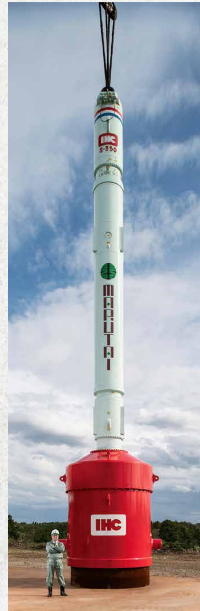
Hydraulic impact hammer S-350 (made in Netherlands)
